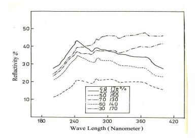
Figure 3: UV Spectral Reflectivity of Deposited Films from Different Pellets
