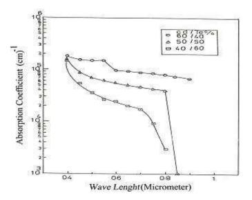
Figure 4: Dependence of Absorption Coefficient on Cd percentage
