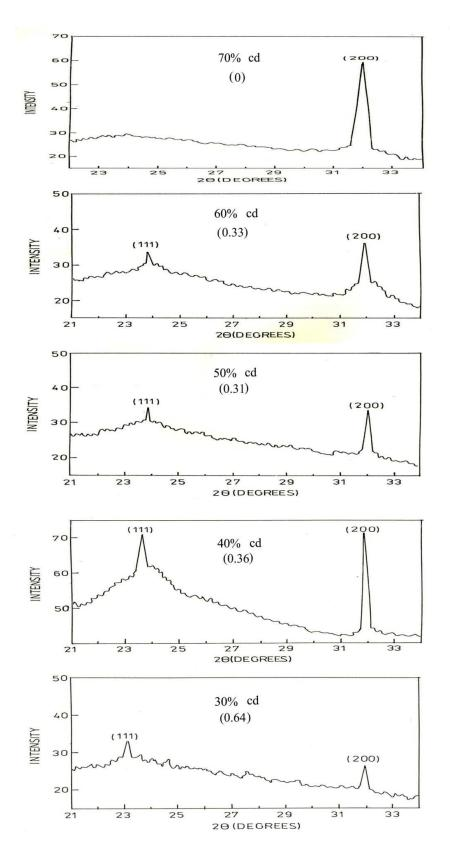
Figure 1: X-ray Diffraction of Deposited thin Films Grown from Pellets of Different cadmium Percentage
