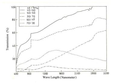
Figure 2: Transmission Spectra of CdTe Films Deposited Film from Different Pellets Percentage
